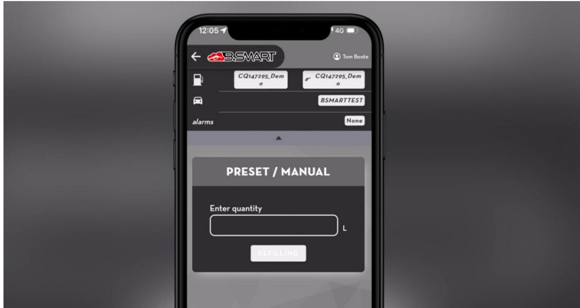
07. Once refuelling has started, the display on the Piusi B.Smart app will count the litres of fuel being dispensed.
