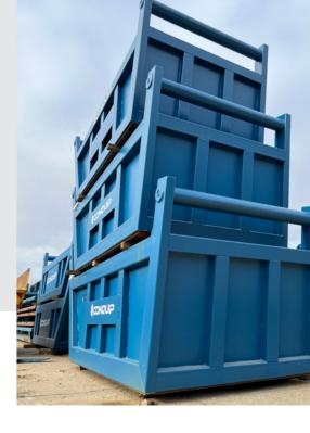
Sometimes referred to as a stone-saver or shingle bin, it is used to transport shingle, saved material for back-fill, and other bulk aggregates across site to the work area.
