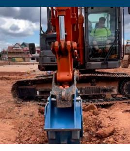
The Excavator Compaction Wheel reduces voids in ground material and increases its density, providing the surface with load-bearing strength.
