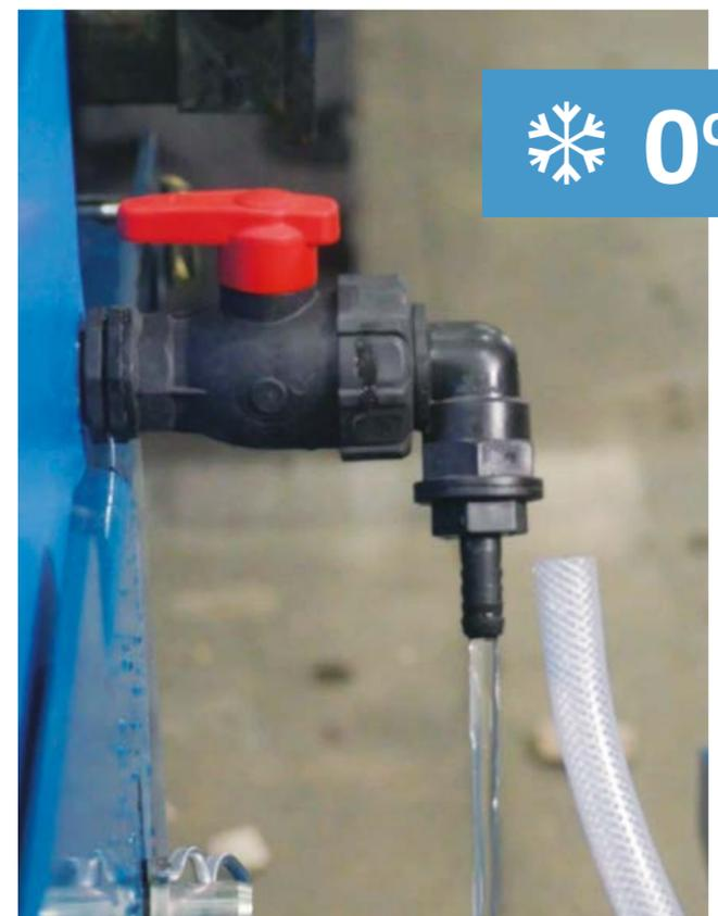
In freezing conditions, remove the hose from the water tap and drain the tank.
