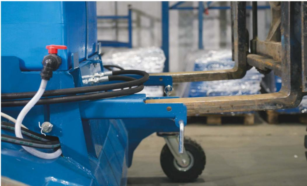
Insert machine (forklift/telehandler) forks into the fork pockets.
