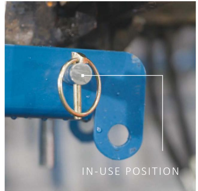
Secure the forks with retaining pins.
