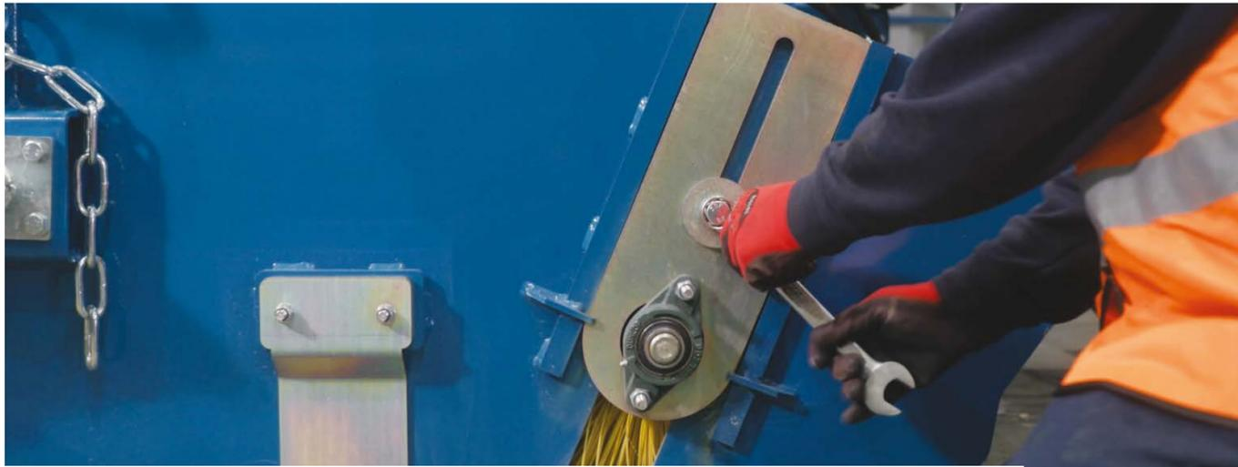
Adjust the height of the main brush with the adjustment bolt, if needed.
